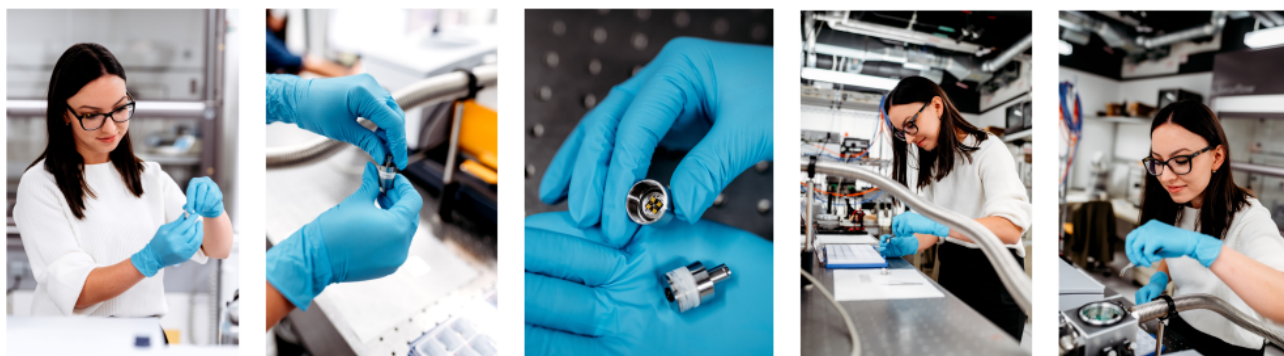
Figure 14: The EMILIE™ chip can be transferred from the Aerosol Flow Adapter to the EMILIE™ infrared analyser without further sample processing.
