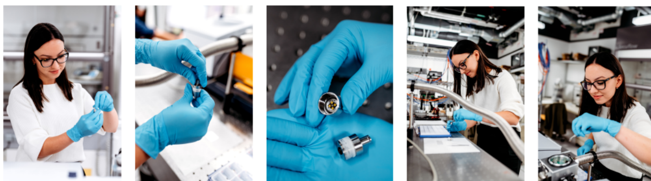
Figure 13: The EMILIE™ chip can be transferred from the Aerosol Flow Adapter to the EMILIE™ infrared analyser without further sample processing.
