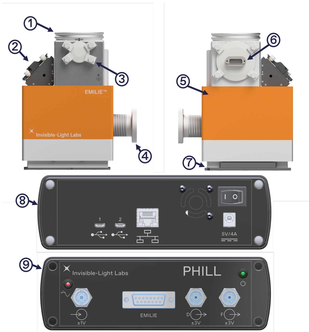
Figure 6: Top: Schematic illustration of EMILIE™'s front (left) and backside (right) highlighting the (1) Vacuum chamber, (2) Kinematic mirror mount, (3) KF25 vacuum flange, (4) Optical port, (5) Purge box with internal optics, (6) Sub-D 15 Pin connector, and (7) Bruker FTIR Quick-Lock plate. Bottom: Schematic illustration of PHILL™'s (8) back panel and (9) front panel.
