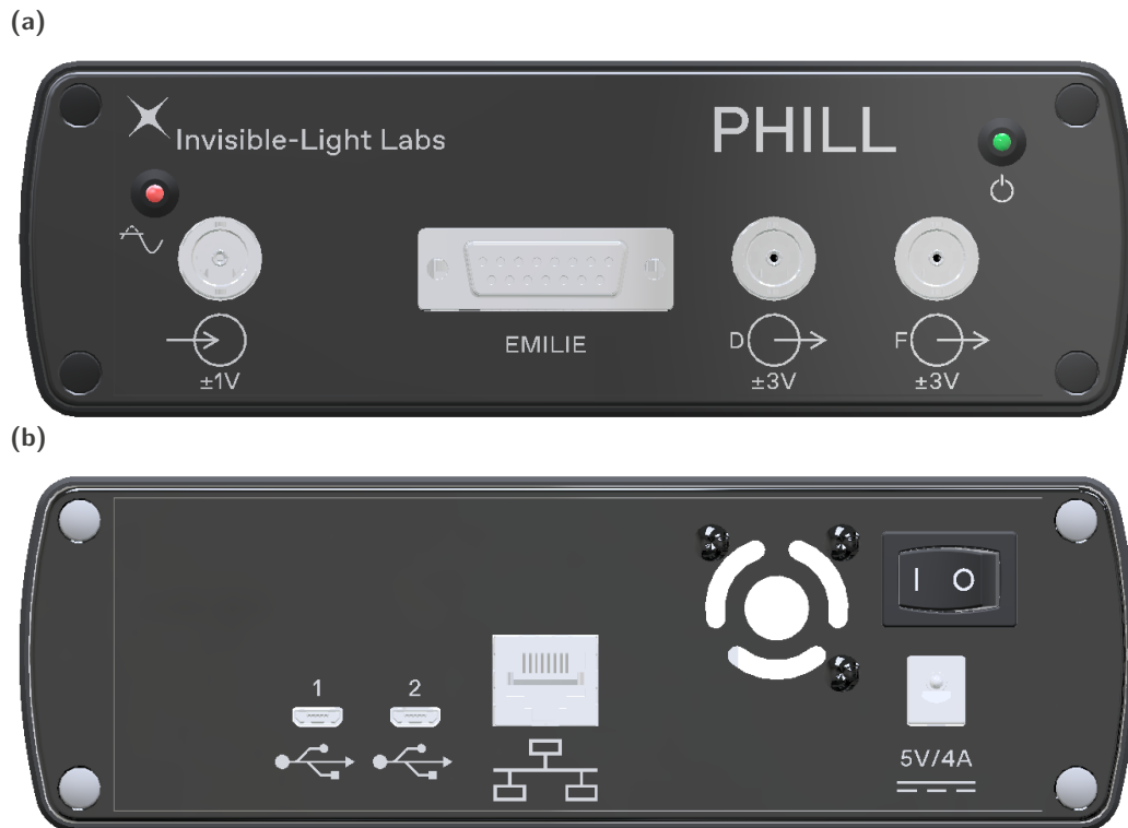
Figure 66: (a) Front plate of PHILL™, (b) Back plate of PHILL™
