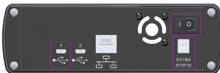
Figure 30: Back panel of PHILL™ highlighting the power switch, micro USB 2.0 port "1", and DC power supply port.
